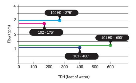
FIGURE 1: Flow Rate vs Depth Apollo-AC 101, 101HD, 102, and 102HD
