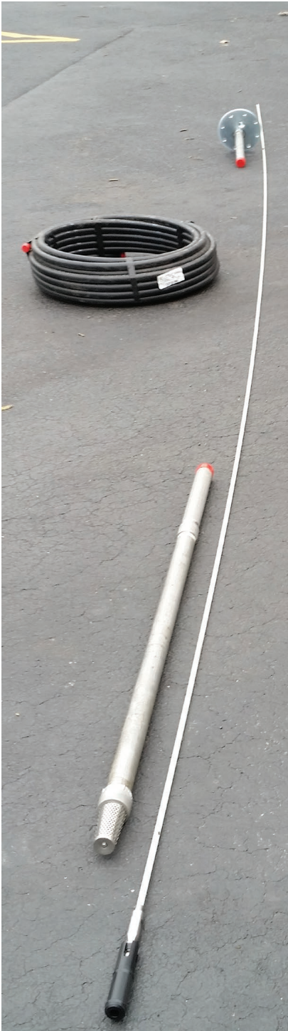
Lay out piston, drive rod, well seal and discharge tee. At left are foot-valve assembly and coiled HDPE riser pipe.
